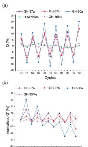
**Fig. 6** (a) Swelling degree and (b) normalised storage modulus of supramolecular hydrogels GH-37a, GH-37c, GH-30a and control hydrogels H-PNiPAAm and GH-35Me. R1-R5 and O1-O5 correspond to the cycle number of reduction and oxidation, respectively.
