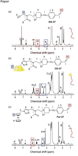
Fig. 2  $\,^{1}$ H NMR spectra of PMOXA macromonomers. (a)  $\,^{1}$ H NMR spectrum of alkyne PMOXA (Alk-37) recorded in CDCl<sub>3</sub>, (b)  $\,^{1}$ H NMR spectrum of CD-PMOXA (CD-37) recorded in DMSO-d<sub>6</sub>, (c)  $\,^{1}$ H NMR spectrum of Fer-PMOXA (Fer-37) recorded in DMSO-d<sub>6</sub>.
