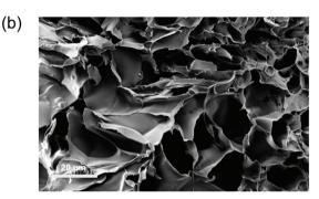
Fig. 5 (a) SEM image of GH-37c in sodium thiosulfate (reduced, scale bar 20 µm), (b) SEM image of GH-37c in hydrogen peroxide (oxidised, scale bar 20 µm).
