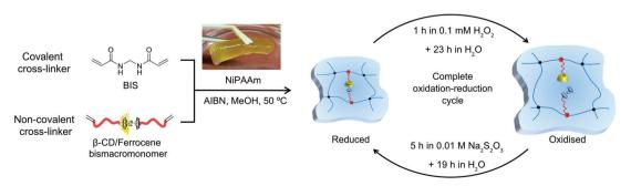
Fig. 4 Chemical structure and synthesis steps of supramolecular redox responsive ferrocene-β-CD hydrogels, including the optimised procedure to achieve fully oxidised and fully reduced hydrogels.
