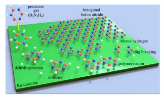
Fig. 1 Schematic illustrating the epitaxial growth of h-BN by chemical vapour deposition: a gaseous precursor (e.g. borazine, B<sub>3</sub>N<sub>3</sub>H<sub>6</sub>) is brought into contact with a (hot) catalyst surface (Ru), triggering the chemical reactions such as breaking of the borazine rings and dehydrogenation, followed by the assembly of the epitaxial overlayer.
