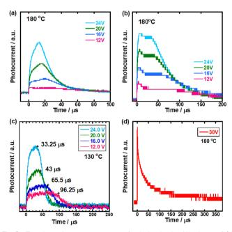
Fig. 2 Transient photocurrent curves for holes in the N\* phase of (a) compound 1 at 180 °C, (b) 2 at 180 °C, (c) 3 at 130 °C, and (d) 4 at 180 °C. The sample thickness was  $4 \mu m$  and the wavelength of the excitation pulse was 356 nm
