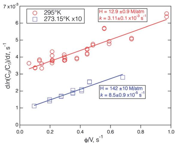
Fig. 7 The results of Henry's law coefficient measurements in DI H<sub>2</sub>O at 295 K, and 273.15 K (enlarged  $\times 10$  on the y-axis). The errors in individual decay rates are smaller than the width of the symbols. The  $H$  and  $k$  values and associated uncertainties were obtained from the fit of the data points to eqn (3).
