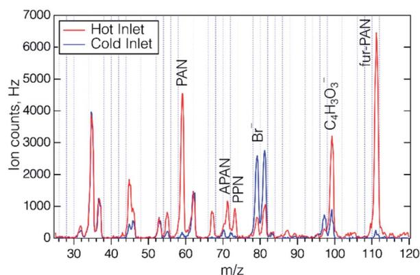
Fig. 2 Mass spectra of the output of the fur-PAN source added to ambient air and measured with the quadrupole I<sup>-</sup> CIMS, through the heated (red) and cold (blue) PAN inlet.
