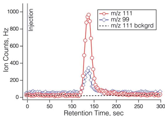
Fig. 4 GC trace during the separation of the effluent of the fur-PAN source on a 2 m Rtx-1 column, 0.53 mm ID, 1.5  $\mu$ m film thickness. The furoate anion ( $m/z$  111) is shown in red and the 4-oxo-2-butenate anion ( $m/z$  99) is shown in blue.
