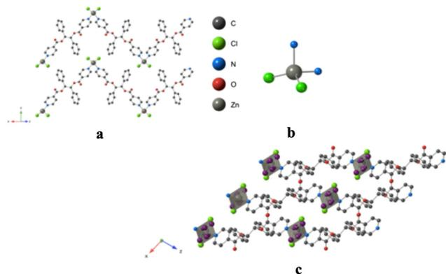
Fig. 4 For  $L\text{-ZnCl}_2$ , portions of the X-ray structure showing a) the formation of the 1D zig-zag type coordination polymer, b) environment around the  $\text{Zn}^{2+}$  cations and c) packing of consecutive networks in the  $xOz$  plane. Disordered chloroform solvent molecules are represented in purple. H atoms are not represented for clarity.
