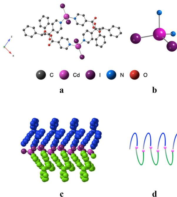
Fig. 5 For  $L\text{-CdI}_2$  a) portion of the X-ray structure of  $L\text{-CdI}_2$  b) environment around the  $\text{Cd}^{2+}$  cations c) the 1D helicoidal coordination polymer, projection in the  $xOz$  plane, and d) schematic representation of the helical 1D structure. H atoms and chloroform solvent molecules are not represented for clarity.
