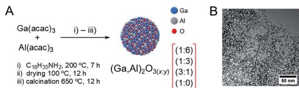
Fig. 1 (A) Synthesis of  $(\text{Ga,Al})_2\text{O}_3(x:y)$  catalysts, where the  $x:y$  index indicates the nominal Ga : Al molar ratio used for the synthesis (1 : 6, 1 : 3, 3 : 1, 1 : 0). (B) A representative TEM image of as-prepared  $(\text{Ga,Al})_2\text{O}_3(1:3)$  nanoparticles in toluene colloidal solution.
