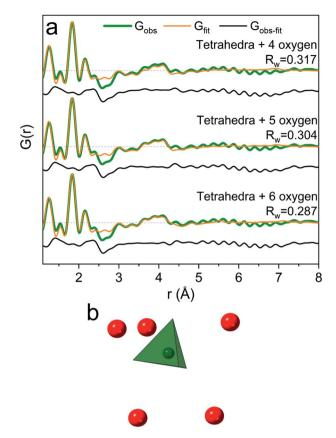
Fig. 9 (a) PDFs of the  $Ga(NO_3)_3$  solution with R=4 modelled with tetrahedrally coordinated Ga<sup>3+</sup> including anions 4, 5 and 6 solvent oxygen atoms. (b) The refined structure with 5 solvent oxygen atoms is shown as the inset with the green tetrahedra representing GaO<sub>4</sub> and oxygen as red spheres.
