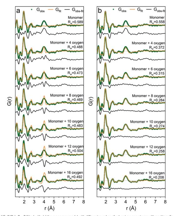
Fig. 5 PDFs of Ga(NO<sub>3</sub>)<sub>3</sub> R = 0 fitted with: (a) the monomer model with different number of solvent oxygen atoms with positions fixed at values in a crystal structure<sup>37</sup> and (b) the same models with refined oxygen positions and a box restraint of  $\pm 0.2$  Å.
