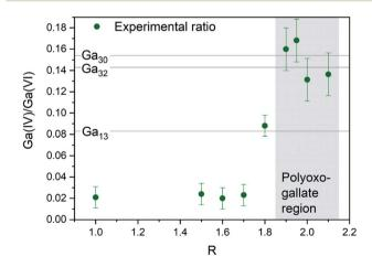
Fig. 7 Experimental ratios of the tetrahedrally to octahedrally coordinated Ga<sup>3+</sup> determined by <sup>71</sup>Ga NMR. The horizontal lines indicate the ratios in the  $Ga_{13}$ ,  $Ga_{30}$  and  $Ga_{32}$  structures at 0.083, 0.154 and 0.143 respectively. The grey area marks the R-region with the highest PDF signal from the polyoxogallate structure.
