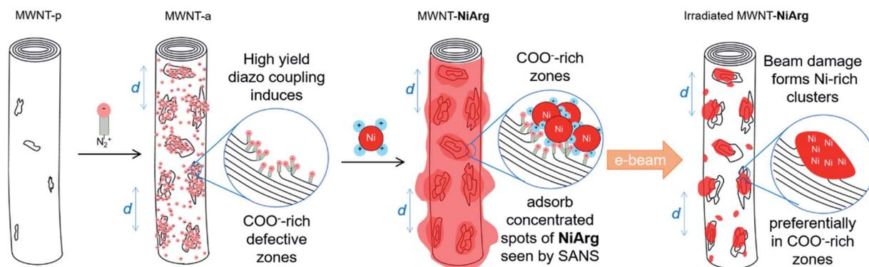
Fig. 6 Scheme of the proposed model for the formation of a cluster distribution of **NiArg** in MWNT-**NiArg** over two steps: diazonaphthoate coupling onto MWNT-p, adsorption of **NiArg** onto MWNT-a. Transformation of the **NiArg** layer following electron-beam exposure is proposed in a third step.
