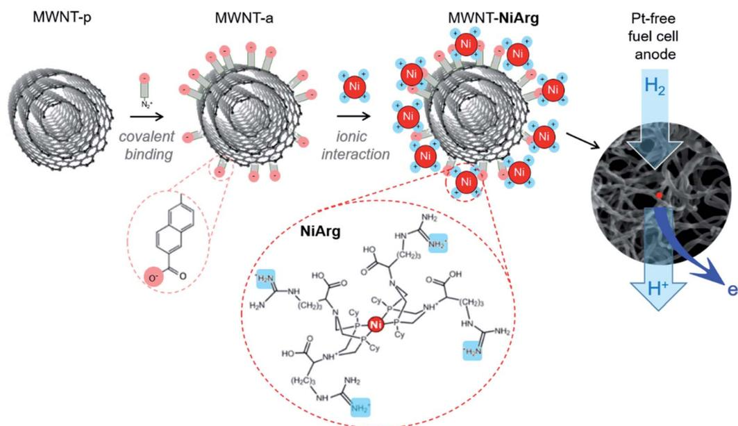
Fig. 1 Scheme of the functionalization of pristine MWNTs (MWNT-p) with naphthoic acid moieties to yield the anionic MWNT-a, and subsequent electrostatic adsorption of **NiArg** catalyst to yield the functional MWNT-**NiArg**, as the catalytic material for platinum-group metal-free fuel cell anodes.
