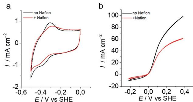
Fig. 2 Electrochemical characterization of MWNT-NiArg anodes without (black) and with (red) Nafion ( $20 \text{ mV s}^{-1}$ ) at room temperature. (a) Cyclic voltammetry (CV) traces in 0.2 M phosphate buffer pH 7 under argon. (b) CV traces at pH 0.3 ( $\text{H}_2\text{SO}_4$  0.5 M) under  $\text{H}_2$ .
