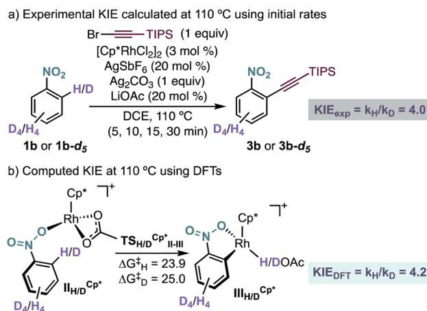
Scheme 6 (a) Experimental and (b) computational KIE for the Rh-catalysed *ortho*-alkynylation of nitrobenzenes **1b** and **1b-d<sub>5</sub>**. Free energies in kcal mol<sup>-1</sup> at 110 °C.
