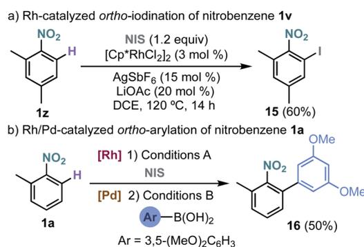
Scheme 5 Rh-catalysed *ortho*-iodination of 2-methylnitrobenzene and one-pot *ortho*-arylation via sequential Rh/Pd catalysis. Conditions A: [Cp\*RhCl<sub>2</sub>]<sub>2</sub> (3 mol%), AgSbF<sub>6</sub> (15 mol%), LiOAc (20 mol%), NIS (1.2 equiv.), DCE, 120 °C, 14 h. Conditions B: Pd(PPh<sub>3</sub>)<sub>4</sub> (5 mol%), DCE, K<sub>2</sub>CO<sub>3</sub>, 60 °C, 14 h.
