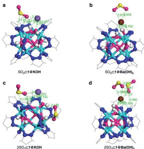
Fig. 6 DFT structure minimization of molecular configuration of one (a and b) and two (c and d) adsorbed SO<sub>2</sub> molecules on 1@KOH (left) and 1@Ba(OH)<sub>2</sub> (right) materials. For sake of clarity, only the region around the metal cluster is shown. Ni (cyan); K (purple); Ba (wine); C (grey); N (blue); O (magenta); H (white); S (yellow). Reprinted (adapted) with permission from ref. 45. Copyright (2017) Springer Nature.
