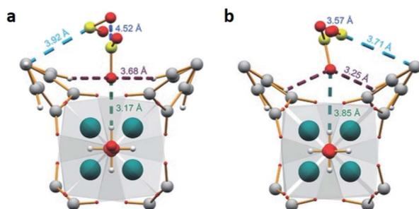
Fig. 3 Binding sites for  $\text{SO}_2$  molecules within MFM-300(In) determined by single-crystal X-ray diffraction (a), and DFT calculations (b). Reprinted (adapted) with permission from ref. 37b. Copyright (2016) John Wiley & Sons.
