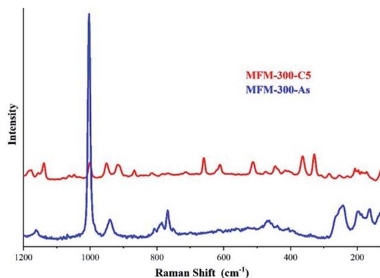
Fig. 11 Raman spectra of MFM-300(Sc) after 5 cycles of H<sub>2</sub>S (red) and as synthesised (blue). The peaks observed in the 350–520 cm<sup>-1</sup> region are associated to the S–S stretching vibrations modes of several polysulphides with various chain lengths. Reprinted with permission from ref. 70. Copyright (2020) American Chemical Society.
