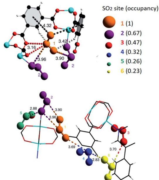
Fig. 1  $\text{SO}_2$  positions within MFM-170 pores obtained from *in situ* single-crystal X-ray diffraction. Purple  $\text{SO}_2$  molecule is located at the thermodynamically strongest binding site. Cu, cyan; C, black; O, red; N, blue. Reprinted (adapted) with permission from ref. 19. Copyright (2019) Springer Nature.
