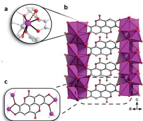
Fig. 12 (a) The coordination environment around Bi<sup>3+</sup>. The bond to a coordinated water molecule is represented as a dashed line. (b and c) Chelation of ellagate ligand toward the bismuth oxo rods. Reprinted (adapted) with permission from ref. 74. Copyright (2020) American Chemical Society.
