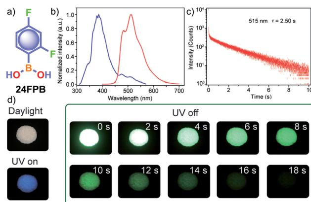
Fig. 3 (a) Chemical structure of **24FPB** and (b) steady-state photo-luminescence (blue line) and phosphorescence (red line) spectra of **24FPB**. (c) Phosphorescence decay profile of the emission band at 515 nm. (d) Photographs of the **24FPB** crystal taken at different time intervals before and after removing the excitation source (a 365 nm UV lamp). Reproduced with permission from ref. 80. Copyright 2019, WILEY-VCH.
