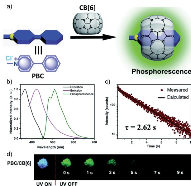
Fig. 7 (a) Schematic illustration of the solid-state supramolecular strategy of PBC and **CB[6]** for URTP. (b) Excitation, emission, and phosphorescence spectra of **PBC/CB[6]** in the solid state. (c) Phosphorescence decay of **PBC/CB[6]** at 510 nm. (d) Photographs of **PBC/CB[6]** powder under 365 nm UV irradiation and at different time intervals after removal of the ultraviolet lamp. Reproduced with permission from ref. 96. Copyright 2019, Royal Society of Chemistry.
