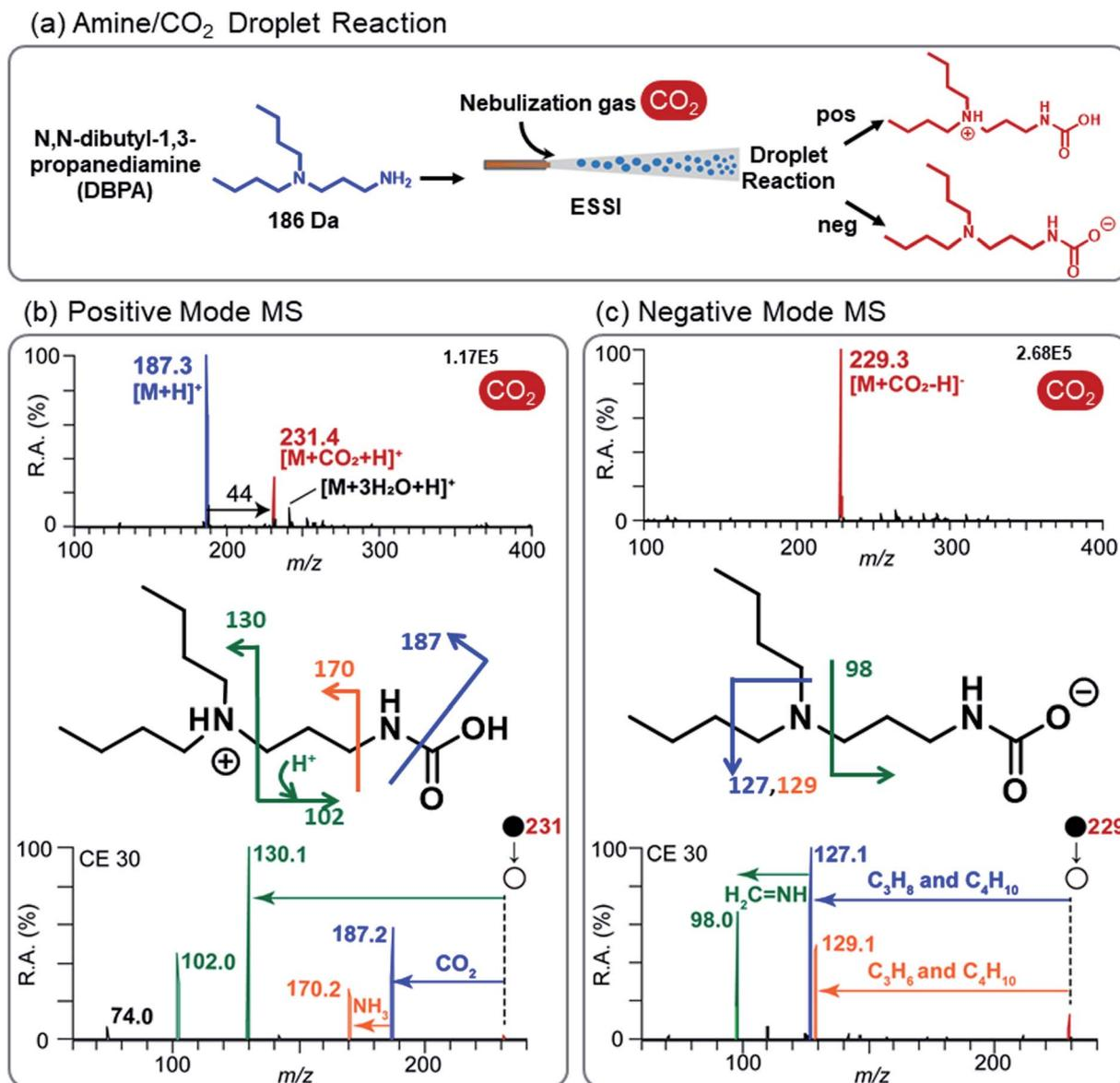
Fig. 1 DBPA/CO<sub>2</sub> droplet reaction by adding CO<sub>2</sub> in the gas phase (a) Droplet reaction of amine/CO<sub>2</sub> conducted by ESSI. (b) Positive and (c) negative mode mass spectra and MS/MS spectra showing fragmentation of protonated and deprotonated DBPA carbamic acid.
