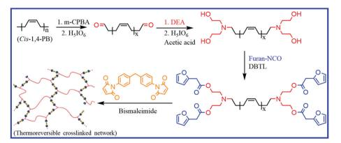
Fig. 5 Schematic representation of the preparation of furan telechelic PB rubber and its DA adduct.<sup>70</sup> Reproduced from ref. 70 with permission from American Chemical Society, copyright 2018.
