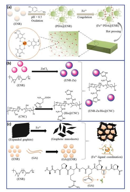
Fig. 15 Schematic representation of the preparation of self-healing ENR via reversible coordinate bonds; (a) catechol-Fe<sup>3+</sup>, (b) histidine-Zn<sup>2+</sup>, and (c) gelatine-Fe<sup>3+</sup>. 96-98 Reproduced from ref. 96 with permission from American Chemical Society, copyright 2017. Reproduced from ref. 98 with permission from American Chemical Society, copyright 2019.
