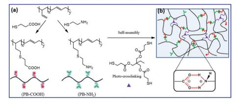
Fig. 8 (a) Schematic representation of the preparation of –COOH and –NH<sub>2</sub> functionalized PB *via* the thiol–ene reaction. (b) The polymer network having both ionic hydrogen bonds and covalent cross-links.<sup>73</sup> Reproduced from ref. 73 with permission from Royal Society of Chemistry, copyright 2015.
