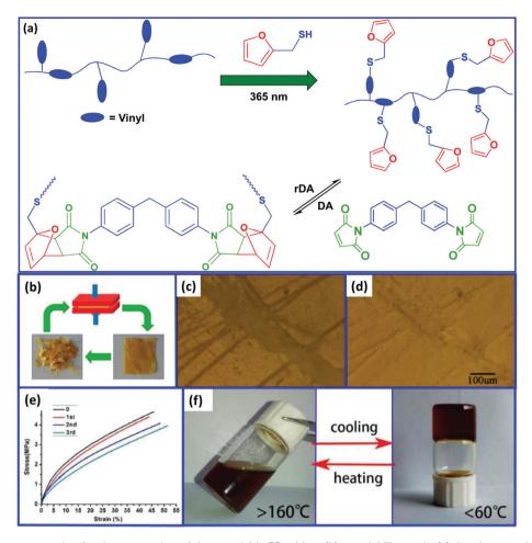
Fig. 4 (a) Schematic representation for the preparation of the recyclable PB rubber, (b) recyclability study, (c) the photograph of the scratched film at room temperature, (d) the photograph of the film after healing at 150 °C, (e) stress-strain curves of the pristine and the recycled samples, and (f) the sol-gel process in dichlorobenzene at different temperatures.<sup>69</sup> Reproduced from ref. 69 with permission from American Chemical Society, copyright 2015.
