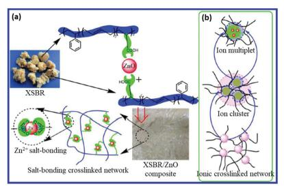
Fig. 9 (a) Schematic representation of network formation by the reaction between carboxyl groups of XNBR and zinc oxide. (b) Schematic for ion multiplet, ion cluster, and ionic crosslinked network.<sup>79</sup> Reproduced from ref. 79 with permission from American Chemical Society, copyright 2016.
