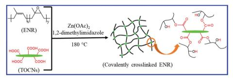
Fig. 18 Schematic representation of the preparation of TOCNs cross-linked ENR *via* the epoxy-acid reaction<sup>112</sup> Reproduced from ref. 112 with permission from Royal Society of Chemistry, copyright 2019.
