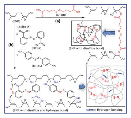
Fig. 17 (a) Schematic representation of the preparation of self-healing ENR having aliphatic disulfide functionality. <sup>106</sup> (b) Self-healing ENR having aromatic disulfide functionality and hydrogen bonding. <sup>107</sup> Reproduced from ref. 106 with permission from Royal Society of Chemistry, copyright 2015. Reproduced from ref. 107 with permission from American Chemical Society, copyright 2019.
