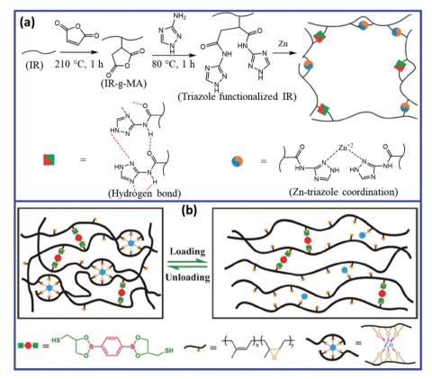
Fig. 16 (a) Schematic representation of the preparation of self-healing IR via a dual dynamic network based on reversible hydrogen and coordinate bond. (b) Self-healing ENR networks with dual dynamic crosslinks of boronic ester bonds and non-covalent  $Zn^{2+}$ –O coordinate bonds. Reproduced from ref. 100 with permission from Royal Society of Chemistry, copyright 2019. Reproduced from ref. 101 with permission from American Chemical Society, copyright 2019.
