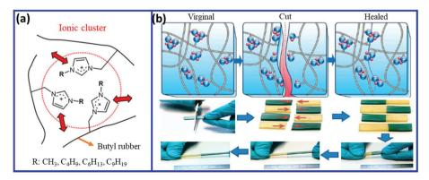
Fig. 20 (a) Schematic representation of the formation of the ionic cluster in the imidazole-modified BIIR.<sup>127</sup> (b) Dissociation and association ionic groups during the self-healing process. <sup>126</sup> Reproduced from ref. 126 with permission from American Chemical Society, copyright 2015. Reproduced from ref. 127 with permission from American Chemical Society, copyright 2017.
