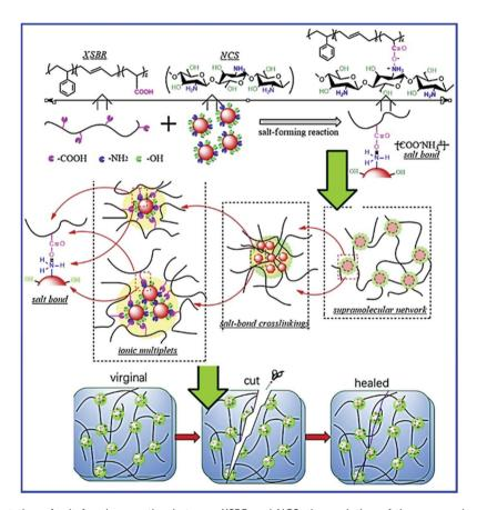
Fig. 10 Schematic representation of salt-forming reaction between XSBR and NCS, the evolution of the supramolecular hybrid network in the XSBR/NCS composites, and self-healing by the reestablishment of ionic bond crosslinking in the supramolecular XSBR network.<sup>80</sup> Reproduced from ref. 80 with permission from Elsevier, copyright 2019.
