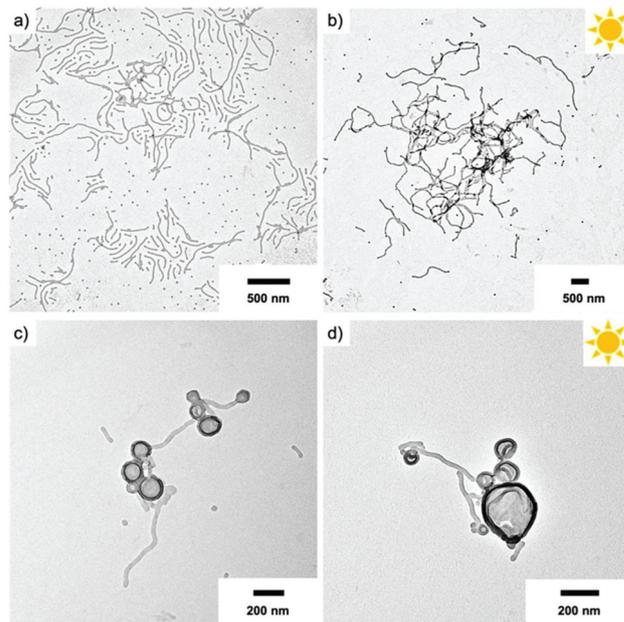
**Fig. 6** Morphologies of PEO<sub>113</sub>-ONB-*b* PS<sub>x</sub> BCPs in water. TEM of P2 cylinder micelles at  $c = 0.1 \text{ mg mL}^{-1}$  before irradiation (a) and after irradiation (b). TEM of P3 vesicles at  $c = 0.1 \text{ mg mL}^{-1}$  before irradiation (c) and after irradiation (d).
