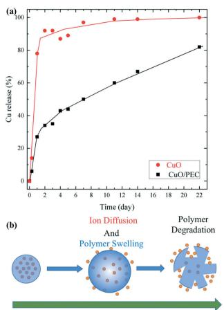
Fig. 6 (a) Cumulative percentage release of Cu versus time from CuO nanopowder and the CuO/PEC NPs, under a constant of pH = 5.5. (b) Schematic of the mechanism of Cu release from the CuO/PEC nanocomposite
