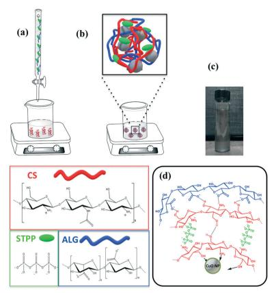
Fig. 1 (a) and (b) Schematic of the preparation of the CuO/PEC nanocomposite with a scheme of its chemical structure; (c) photograph of the CuO/PEC solution; (d) scheme of the CuO/PEC structure and interactions.
