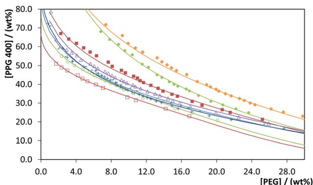
Fig. 1 Phase diagrams for the systems composed of PPG 400 + PEG + H<sub>2</sub>O with PEGs of different molecular weights: PEG 600 (◆); PEG 1000 (●); PEG 2000 (■); PEG 4000 (△); PEG 6000 (×); PEG 8000 (+); PEG 10 000 (○); PEG 20 000 (□). The lines correspond to the respective correlations (detailed in the ESI†).
