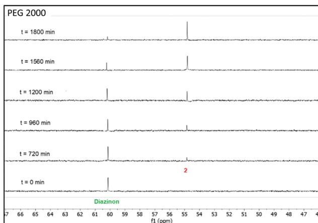
Fig. 6 Stacked  $^{31}\text{P}$ -NMR spectra for the nucleophilic degradation of diazinon with piperidine performed in a mixture of 35 wt% PPG 400 + 15 wt% PEG 2000 + 50 wt%  $\text{H}_2\text{O}$  at 298 K.
