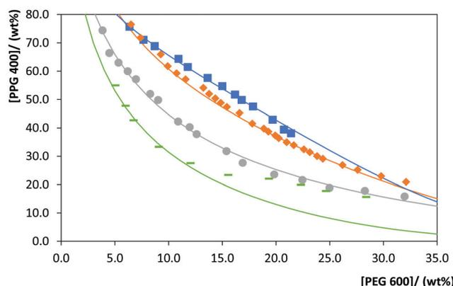
Fig. 2 Phase diagrams for the system composed of PPG 400 + PEG 600 + H<sub>2</sub>O at different temperatures: 288 K (■); 298 K (◆); 308 K (●); 313 K (×). The lines correspond to the respective correlations (detailed in the ESI†).
