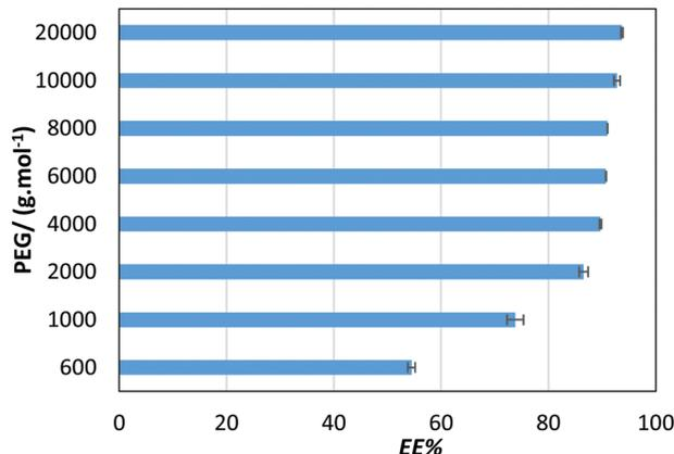
Fig. 4 Extraction efficiencies (*EE*%) of diazinon to the PPG-rich phases in ABSs formed by 35 wt% PPG 400 + 15 wt% PEG + 50 wt% H<sub>2</sub>O at 313 K.
