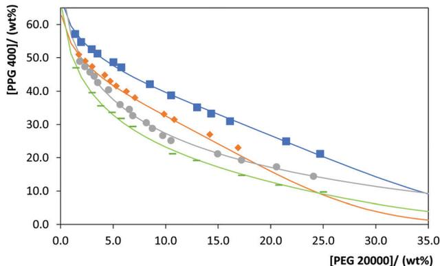
Fig. 3 Phase diagrams for the system composed of PPG 400 + PEG 20 000 + H<sub>2</sub>O at different temperatures: 288 K (■); 298 K (◆), 308 K (●); 313 K (×). The lines correspond to the respective correlations (detailed in the ESI†).
