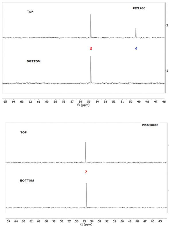
Fig. 8  $^{31}\text{P}$ -NMR spectra of both phases of the ABS composed of 35 wt% PPG 400 + 15 wt% PEG (600 and 20 000) + 50 wt%  $\text{H}_2\text{O}$  used as - reaction media of nucleophilic degradation of diazinon with piperidine.
