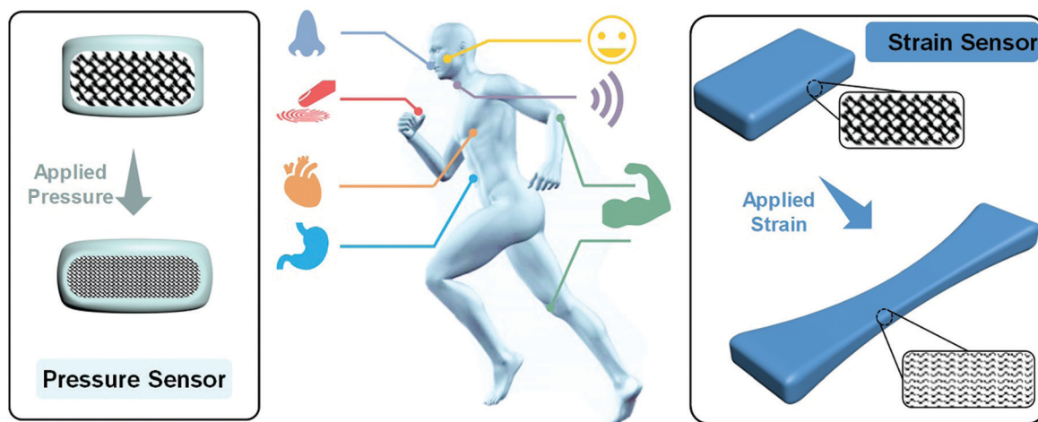
Fig. 1 Schematic illustration of potential applications of flexible pressure and strain sensors for implantable and wearable devices.
