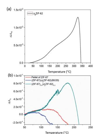
Fig. 6 Thermo-mechanical properties. Linear thermal expansion of (a)  $a_{\rm g}$ ZIF-62 and (b) ZIF-67 series measured by TMA.
