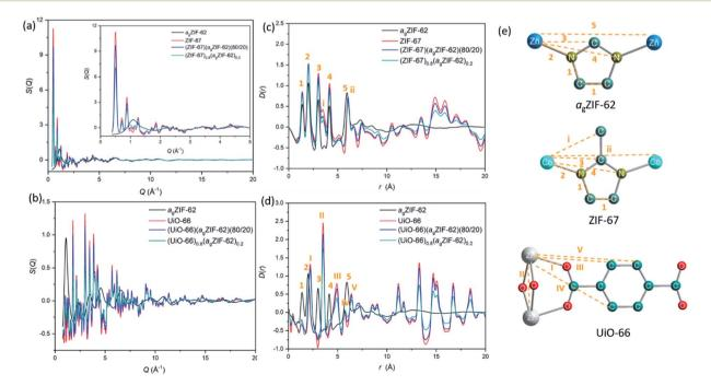
Fig. 2 X-ray total scattering. (a and b) structure factors, S(Q), of  $a_gZIF-62$ , ZIF-67, UIO-66 physical mixtures and CGCs. (c and d) Corresponding pair distribution functions, D(r). (e) Scheme of peak assignment of PDF patterns. Zn, blue; C, dark green; N dark yellow; Co, light blue; Zr, grey; O, red; H, omitted for clarity.
