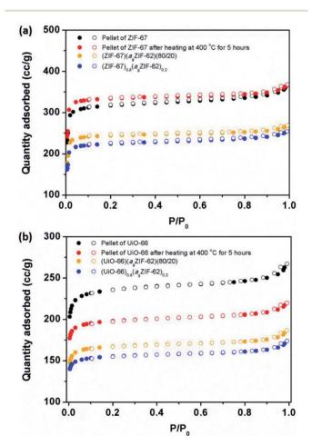
Fig. 5 Gas sorption.  $N_2$  gas isotherms at 77 K of (a) ZIF-67 series, and (b) UiO-66 series. Solid circles represent adsorption, and hollow circles represent desorption.
