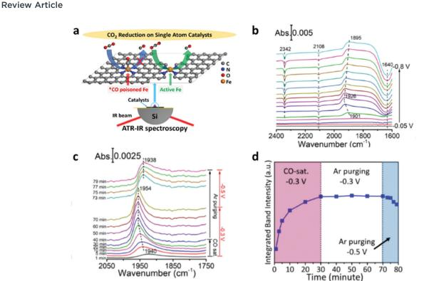
Fig. 23 (a) Scheme of the setup. (b) Real-time ATR-IR spectra recorded while stepping the potential of the Fe-N-C-loaded Au/Si prism in the CO<sub>2</sub>-saturated 0.5 M KHCO<sub>3</sub>. (c) Real-time IR spectra and (d) the evolution of the integrated \*CO band intensity when switching the CO/Ar atmosphere and potential. IR references were taken at 0 V for panel (b) and 0.1 V for panel and (c). Adapted with permission from ref. 339. Copyright 2019 American Chemical Society.
