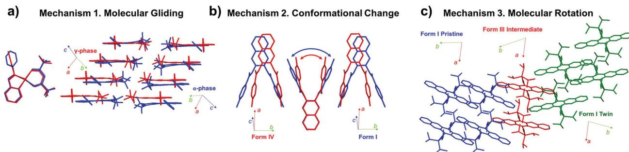
Fig. 6 Molecular mechanisms found in martensitic transitions, showing (a) molecular gliding,<sup>40</sup> (b) conformational change,<sup>46</sup> and (c) molecular rotation.<sup>57</sup> Examples of each mechanism are depicted by structural changes in #5 (CCDC 103651 and 1013657), #8 (CCDC 1583404 and 1583405), and #13 crystals (CCDC 1970910 and 1991343) of Fig. 2, respectively.
