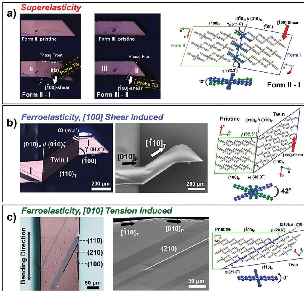
Fig. 15 (a) Superelasticity of #13 crystal in Fig. 2 based on  $[100]$  shear induced Form II–I and Form III–II transition. (b) Ferroelasticity of #13 crystal based on  $[100]$  shear and (c)  $[010]$  tension. Adapted with permission from ref. 57, copyright 2020 John Wiley & Sons, Inc.
