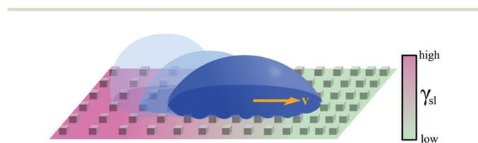
Fig. 6 Simplified schematic of droplet transport due to gradients in surface texture. Space-varying structural features can lead to directional droplet transport at a velocity  $\mathbf{v}$  towards areas of lower surface energy by influencing the contact angle that the droplet assumes on it. For example, an array of pillars of varying width and separation can induce a droplet to move towards areas of larger surface coverage when contact angle hysteresis is overcome.<sup>7</sup>
