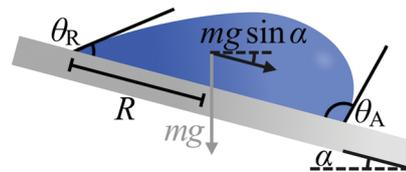
**Fig. 3** Hindrance to droplet motion due to contact angle hysteresis. A droplet of radius  $R$  on an incline will start moving only when gravity deforms it past the range of acceptable contact angles allowed by its hysteresis. Practically, at a given angle  $\alpha$ , motion will take place only when the advancing contact angle  $\theta_A$  at the front of the droplet and the receding contact angle  $\theta_R$  at its rear take values other than those allowed by contact angle hysteresis.
