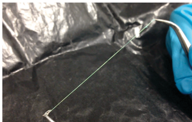
Fig. 8 A long (~20 cm) sample of a PI fibre filled with a mixture of 25% w/w ZLI-3786 in RO-TN 651, viewed under ambient room lighting.
