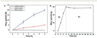
Fig. 6 (a) Photocatalytic activities for nitrogen fixation of the assynthesized  $MoO_{3-x}$  nanobelts under LED light irradiation with various wavelengths; (b) control experiment in N2 and Ar gas in succession for photocatalytic nitrogen fixation (light source: 300 W xenon lamp).
