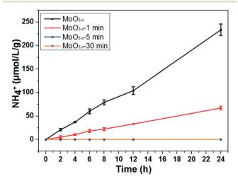
Fig. 4 Photocatalytic experiments for nitrogen fixation of the assynthesized and annealed  $MoO_{3-x}$  nanobelts (light source: 300 W xenon lamp; photocatalyst: 0.05 g; solution: 100 ml of pure water. The error bar results came from photocatalytic experiments of the same samples performed three times.)
