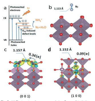
Fig. 8 (a) Electron transfer processes during O<sub>VS</sub>-mediated nitrogen fixation. (b) N2 adsorbed on the pristine surface; (c) terminal side-on adsorption on (001) and (d) end-on bridging adsorption on (100) for N<sub>2</sub> (yellow means increasing charge and blue means decreasing charge).
