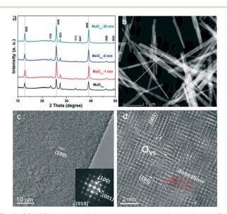
Fig. 1 (a) XRD patterns of the as-synthesized and annealed  $MoO_{3-x}$ nanobelts for various times; (b) HAADF STEM image of the overall morphology of the  $MoO_{3-x}$  nanobelts; (c) HRTEM image of  $MoO_{3-x}$  with the insert showing the electron diffraction pattern; (d) atomic scale HAADF image showing the ordered oxygen vacancies at the (001) & (100) planes.
