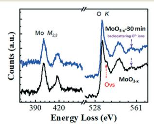
Fig. 2 EELS analysis of the as-synthesized  $MoO_{3-x}$  and  $MoO_{3-x}$  after 30 min annealing in air atmosphere.
