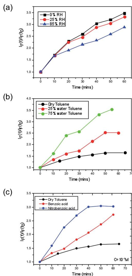
Fig. 3 Superoxide yield plots for  $\text{CH}_3\text{NH}_3\text{PbI}_3$  where (a) demonstrates the effect on the yield via pre-treating the film under no moisture, 25% RH and 85% RH, (b) demonstrates the effect of increasing water content in the toluene solution that houses the superoxide reactive probe and (c) shows the impact of acid strength on the superoxide yield, where benzoic acid and nitrobenzoic acid are doped into the toluene solution.
