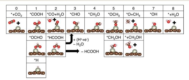
Fig. 3 Key reaction intermediate species for the  $CO_2$  reduction reaction. The numbers on top of each column are the numbers of protonelectron pairs (H<sup>+</sup> + e<sup>-</sup>) transferred to CO<sub>2</sub>.
