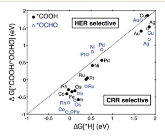
Fig. 2 Free energy change of the first protonation step in the CO<sub>2</sub> reduction reaction (CRR) and H<sub>2</sub> evolution reaction (HER) on the various SACs. Catalysts below the dotted parity line are CRR selective.
