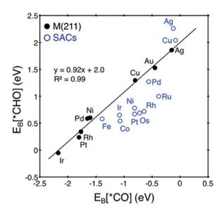
Fig. 5 Correlation between  $E_{\rm B}|^*{\rm CO}|$  and  $E_{\rm B}|^*{\rm CHO}|$  for transition metal (211) surfaces (black) vs. SACs (blue). The conventional scaling relation for M (211) is broken in the case of SACs. We note that Au@dv-Gr is not shown since it does not bind \*CO.
