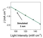
Fig. 3 Photocurrent density recorded at increasing illumination intensity using a CoP-GaP working electrode polarized at 0 V vs. RHE.
