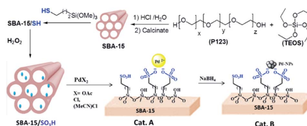
Fig. 24 Schematic representation of the catalysts preparation. Reprinted from ref. 122 with permission of Elsevier.
