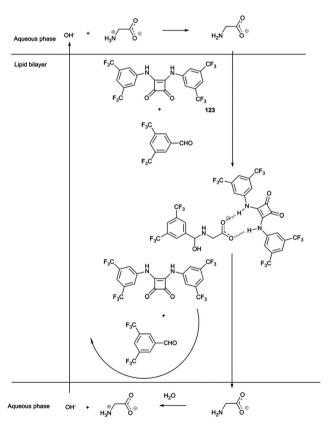
Scheme 1 Proposed mechanism for glycine transport facilitated by compound **123** and 3,5-bistrifluoromethylbenzaldehyde forming a three-component assembly involving hemiaminal formation. Alternatively imine formation is possible. OH<sup>-</sup> transport is facilitated by compound **123** which is not shown.
