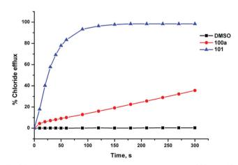
Fig. 25 Chloride efflux mediated by unsubstituted receptors 100a and 101 (2 mol% with respect to lipid) from unilamellar POPC vesicles containing 489 mM NaCl buffered to pH 7.2 with 5 mM sodium phosphate salts. The vesicles were suspended in 489 mM NaNO<sub>3</sub> buffered to pH 7.2 with 5 mM sodium phosphate salts. At the end of the experiment the vesicles were lysed with detergent in order to calibrate 100% chloride release. Each point represents the average of three trials.
