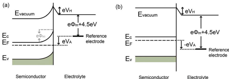
Fig. 5 Effect of applying a bias voltage ( $V_A$ ) to an n-type semiconductor photoelectrode.  $V_H$  is the potential drop across the Helmholtz layer.  $\Phi_m$  is the work function of the metal.  $\Phi_{sc}$  is the potential drop across the space charge region. Reproduced from ref. 3 with permission of Springer Science+Business Media, LLC.
