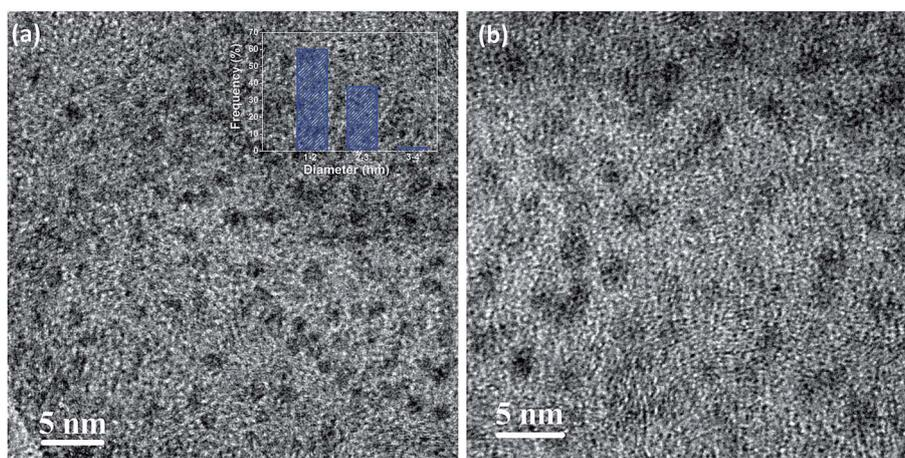
Fig. 1 (a) Low and (b) high resolution TEM images of wsCQDs; inset (a) corresponding size distribution histogram.
