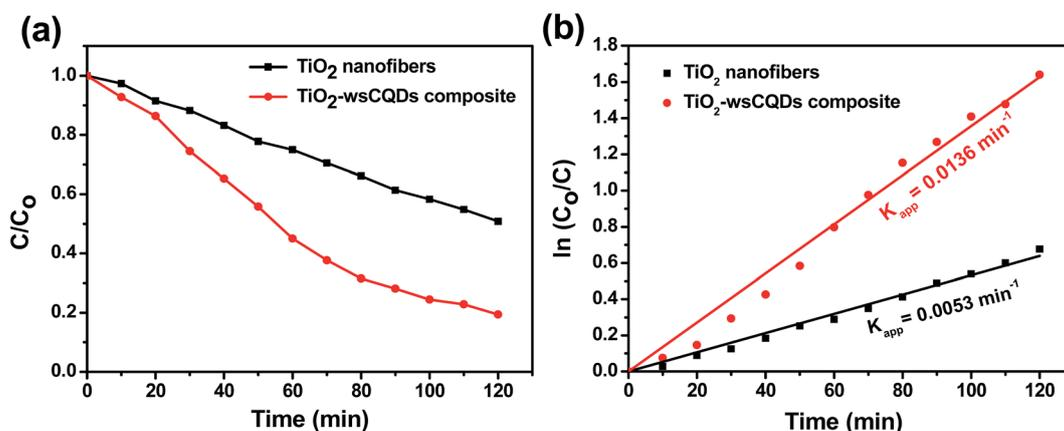
Fig. 7 (a) Photocatalytic degradation of MB in presence of  $\text{TiO}_2$  nanofibers and  $\text{TiO}_2$ -wsCQDs composite under UV light irradiation and (b) photocatalytic reaction kinetics of MB degradation in presence of  $\text{TiO}_2$  nanofibers and  $\text{TiO}_2$ -wsCQDs composite.
