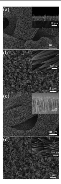
Fig. 3 Typical SEM images of (a), (b) Co<sub>2</sub>(OH)<sub>2</sub>(CO<sub>3</sub>)<sub>2</sub> precursor film and (c), (d) Co<sub>3</sub>O<sub>4</sub> nanowire array grown on nickel foam (side view of the arrays and magnified top view presented in insets).
