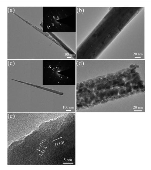
Fig. 4 TEM images of (a), (b) the Co<sub>2</sub>(OH)<sub>2</sub>(CO<sub>3</sub>)<sub>2</sub> nanowire and (c), (d) Co<sub>3</sub>O<sub>4</sub> nanowire; (e) HRTEM image (SAED patterns of the nanowires presented in inset).
