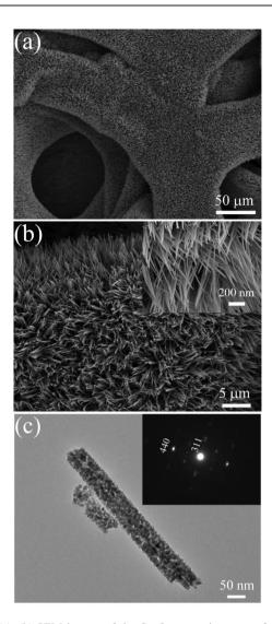
**Fig. 7** (a), (b) SEM images of the Co<sub>3</sub>O<sub>4</sub> nanowire array after cycling for 4000 cycles; (c) a TEM image of the Co<sub>3</sub>O<sub>4</sub> nanowire after cycling for 4000 cycles (SAED pattern in inset).
