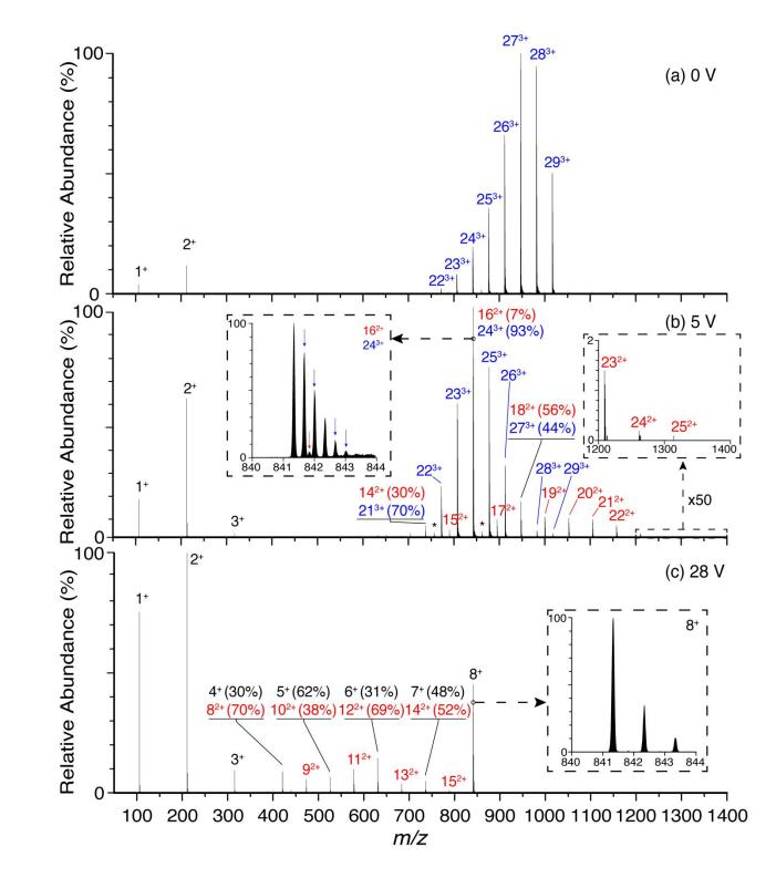
**Figure 3.** Collision induced dissociation spectra of  $29^{3+}$  at collision voltages of (a) 0 V, (b) 5 V and (c) 28 V. Protonated octamer abundance is a maximum at 28 V collision voltage. Peaks
