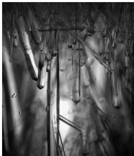
Figure 1. Crystals of the two forms of compound 1 . Above: orthorhombic form 1o , part of the crystal actually measured (max. linear dimension ca. 0.4 mm). Below: tetragonal form 1t as grown in the test-tube with pentane precipitant (total width ca. 2 mm).
