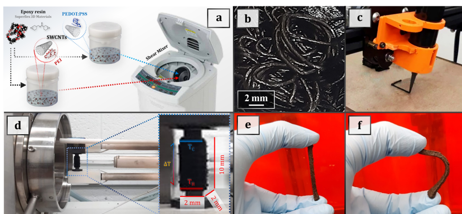
Fig. 1 Thermoelectric paste production process. (a) The dispersion process of the SWCNTs using a shear-mixer, (b) the produced p-type SWCNT/epoxy-based dispersion after extrusion printing, (c) the additive manufacturing process of thermoelements, (d) the thermoelectric characterization of the 3D-printed materials, and (e) and (f) the flexibility of the SWCNT/epoxy-based 3D-printed TE material after curing.
