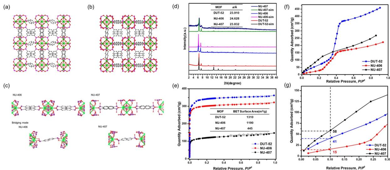
**Fig. 1** Single-crystal structures of (a) NU-406 and (b) NU-407, (c) bridging modes of ligands in NU-406 and NU-407, and (d) powder XRD pattern of DUT-52, NU-406 and NU-407 (color code for atoms: zirconium (green), phosphor (purple), carbon (grey), and oxygen (red)). (e)  $\text{N}_2$  sorption at 77 K of DUT-52, NU-406 and NU-407. (f) Water sorption at 298 K of DUT-52, NU-406 and NU-407 and (g) the zoomed-in view of the low relative pressure region.
