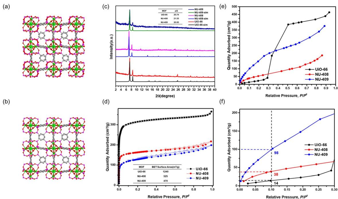
Fig. 2 Simulated structure of (a) NU-408 and (b) NU-409 (color code for atoms: zirconium (green), phosphor (purple), carbon (grey), and oxygen (red)). (c) Powder XRD pattern of UiO-66, NU-408 and NU-409 and their unit cell parameters. (d)  $\text{N}_2$  sorption at 77 K of UiO-66, NU-408 and NU-409. (e) Water sorption at 298 K of UiO-66, NU-408 and NU-409 and (f) the zoomed-in of the 0–0.3  $P/P^0$  range.
