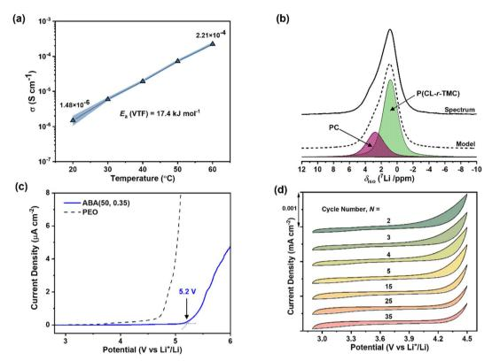
Fig. 3 (a) Temperature-dependence of ionic conductivity for ABA (50, 0.35)/17 wt% LiTFSI. (b) Solid-state  $^{7}$ Li NMR spectrum with peak deconvolution to PC and P(CL-r-TMC) phases. (c) Oxidative stability vs. Li metal and stainless-steel counter electrode measured by LSV at 60 °C, 0.1 mV s $^{-1}$  scan rate. (d) CV at 0.5 mV s $^{-1}$  scan rate recorded over 35 cycles.
