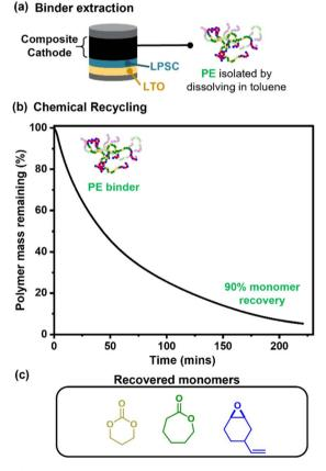
Fig. 6 Chemical recycling of the polymer electrolyte binder, catalysed by  $\rm Zn(Oct)_2/\rm GEO~([Zn(Oct)_2]_0:[\rm GEO]_0:[\rm polymer]_0=1:1.13:1000)$  at 200 °C. Monomers were recovered by distillation under 1 mbar pressure, with the mixture heated to 200 °C. (a) Schematic depicting how the polymer binder can be recovered from the cell. (b) Polymer degradation vs. time, throughout the chemical recycling process. (c) The monomers recovered in the chemical recycling process.
