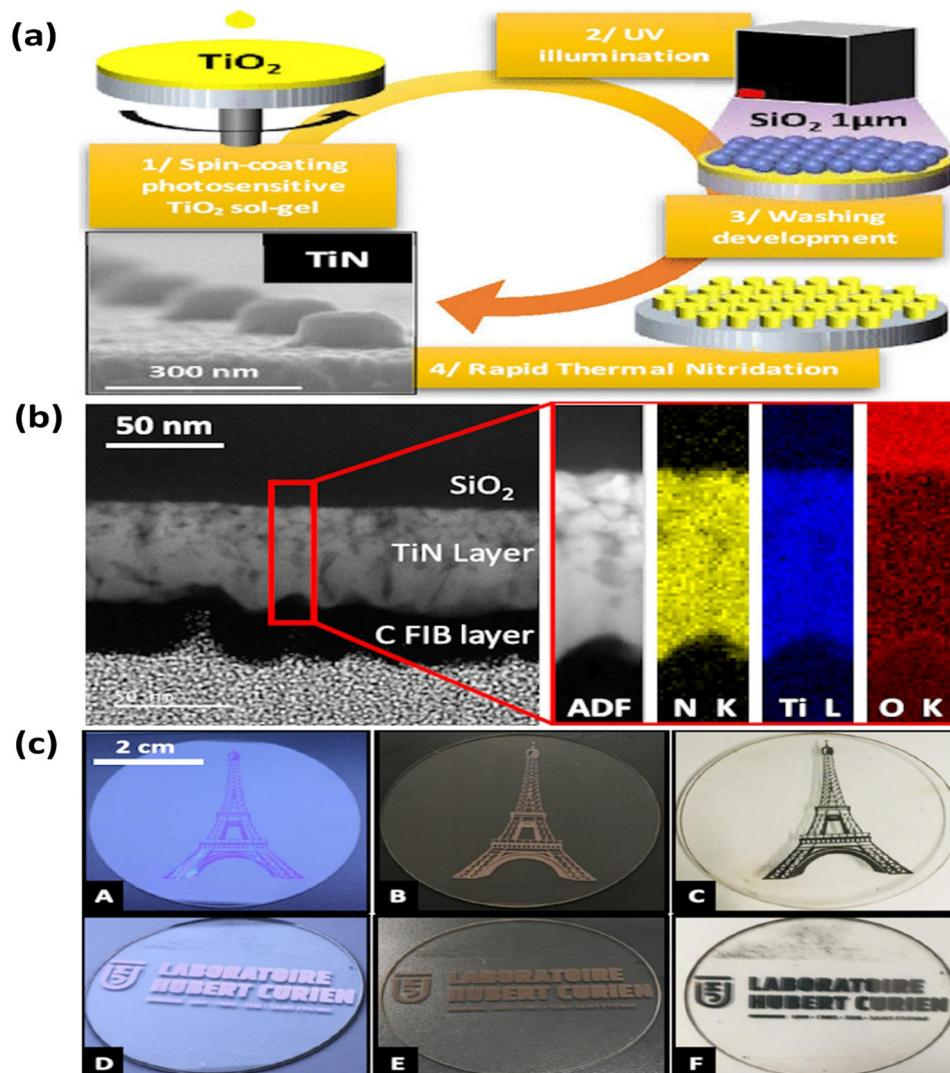
Fig. 8 (a) Scheme for the preparation; (b) cross-sectional HRTEM of the TiN thin film, annular dark field (ADF), and element mapping images for the N, Ti, and O; (c) photographs of structured  $\text{TiO}_2$  thin films after UV exposure (A) and (D), after nitridation (B) and (E) and in transmission (C) and (F) elements in the TiN layer (reproduced from ref. 109 with permission).
