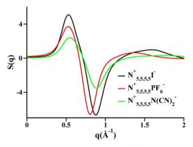
Fig. 4 The cation head—anion subcomponent of S(q),  $S^{H-A}(q)$ , for different ILs in the liquid state. The cation is always the same in this figure, but peaks and antipeaks in the graph are universal for a multitude of ILs having tails long enough to elicit at least some apolar segregation. Reprinted<sup>15</sup> (adapted) with permission from J. Phys. Chem. Lett., 2013, 4(1), 105-110. Copyright 2013 American Chemical Society.
