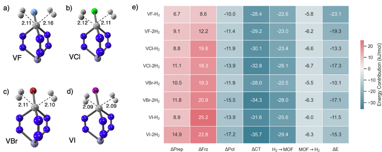
Fig. 13 Multiple H 2 ligations in V(II)-X-MFU-4l, (X = F, Cl, Br, I) (a)–(d) and EDA of the quite wide range of adsorption behaviour as a function of the halide counterion (e). Dative effects, particularly forward donation, dominate the binding energy. Distances are reported in Å, and energy contributions in kJ mol -1 in (e).
