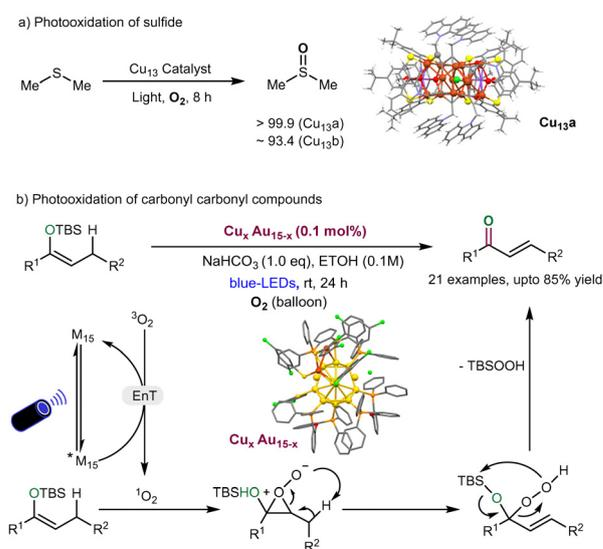
Fig. 7 (a) Quasi-structurally isomeric  $\text{Cu}_{13}$  NCs catalyzed photocatalytic sulfoxidation of sulfides. (b) Photo-oxidation of carbonyl compound derivatives by  $\text{Cu}_x\text{Au}_{15-x}$  NCs.
