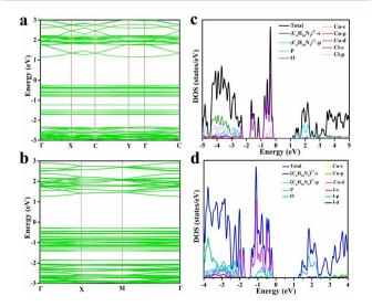
Fig. 4 Band structures of (a) DPCu<sub>4</sub>Cl<sub>6</sub> SCs and (b) DPCu<sub>4</sub>l<sub>6</sub> SCs. Total and orbital-projected DOSs for (c) DPCu<sub>4</sub>Cl<sub>6</sub> SCs and (d) DPCu<sub>4</sub>l<sub>6</sub> SCs.
