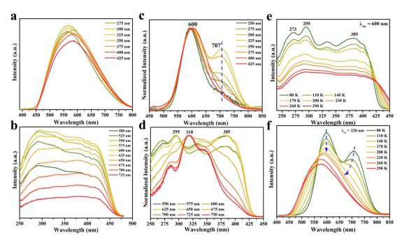
Fig. 3 Excitation and emission-wavelength dependent (a) PL and (b) PLE spectra of DPCu<sub>4</sub>I<sub>6</sub> SCs at RT. Normalized excitation and emission-wavelength dependent (c) PL and (d) PLE spectra of DPCu<sub>4</sub>I<sub>6</sub> SCs at 80 K. Temperature-dependent (e) PLE and (f) PL spectra of DPCu<sub>4</sub>I<sub>6</sub> SCs.
