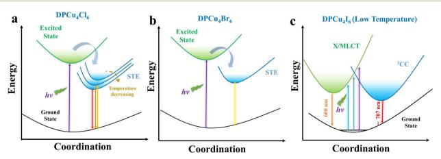
Fig. 5 Schematic of the photophysical processes in (a) DPCu<sub>4</sub>Cl<sub>6</sub>, (b) DPCu<sub>4</sub>Br<sub>6</sub>, and (c) DPCu<sub>4</sub>l<sub>6</sub> SCs.
