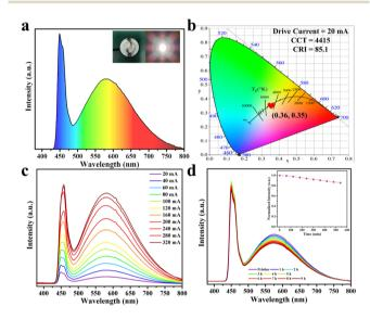
Fig. 6 (a) Luminescence spectrum of the WLED device fabricated with DPCu $_4$ l $_6$  powder excited with a 450 nm blue light chip. The insets show photographs of a WLED with power off (left) and power on (right). (b) CIE coordinate of the WLED. (c) Drive current-dependent electroluminescence spectra. (d) Emission stability of the WLED at 20 mA driving current for 9 h. The inset shows the integrated luminous intensity of the WLED device working over different periods.
