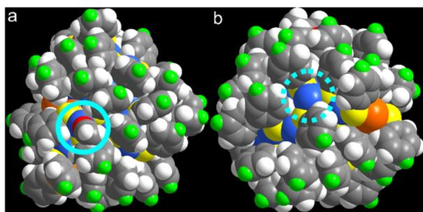
**Fig. 3** Au<sub>41</sub>Cu<sub>33</sub>(RS)<sub>40</sub>(MeCN) cluster in space-filling mode showing the presence of uncoordinated atoms on the surface. Color codes for atoms: orange spheres, Au; blue spheres, Cu; magenta spheres, P; purple spheres, Sb; bright green spheres, F; and grey spheres, C. All hydrogen atoms are omitted for clarity.
