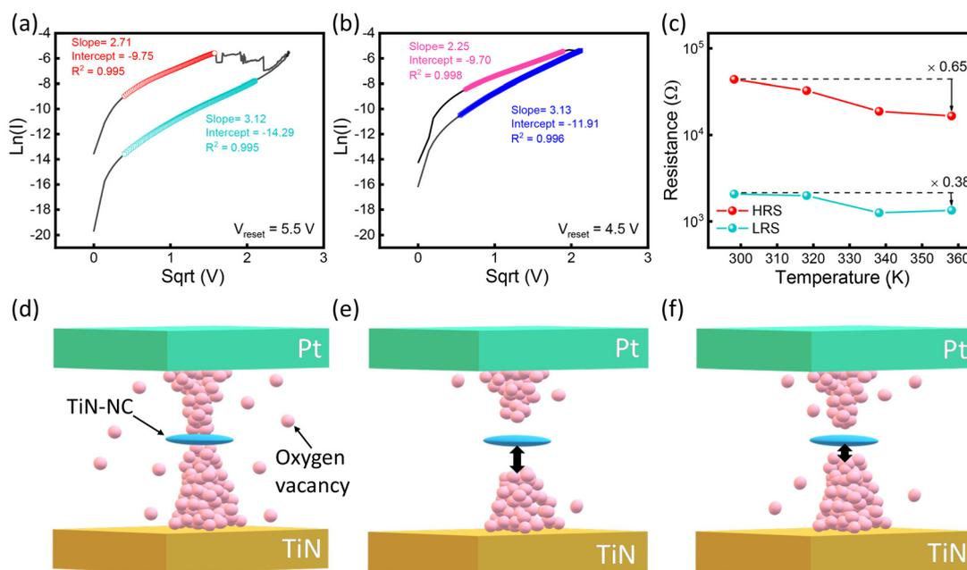
**Fig. 7** Current fitting of the HRS and LRS with different reset voltages: (a) 5.5 V and (b) 4.5 V. (c) Temperature dependence of the resistance state. Schematic diagram illustrating the conduction mechanism: (d) set process and multilevel switching process mechanism with reset voltages of (e) 5.5 V and (f) 4.5 V.
