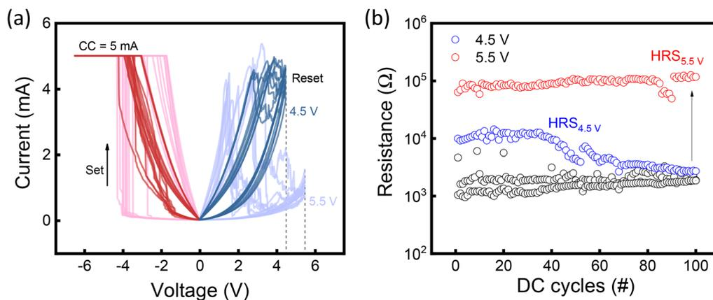
Fig. 6 Multilevel characteristics of Pt/Ti/HfO<sub>x</sub>/TiN-NCs/HfO<sub>x</sub>/TiN VRRAM: (a) DC switching *I*-*V* curves and (b) DC endurance (100 repeated sweeps).
