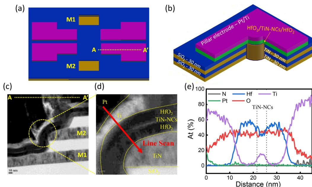
**Fig. 1** 3D schematic diagram of  $4 \times 2 \times 2$  vertical resistive random-access memory (VRRAM): (a) top view and (b) bird's eye view. (c) Cross-sectional TEM image and (d) enlarged switching area of  $\text{Pt}/\text{Ti}/\text{HfO}_x/\text{TiN-NCs}/\text{HfO}_x/\text{TiN}$  VRRAM (red line: EDS line scan). (e) Energy-dispersive spectroscopy (EDS) line analysis of VRRAM cells.
