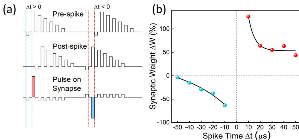
**Fig. 10** (a) Pulse scheme for pre-spike, post-spike, and effective pulse on synapses. (b) Spike-timing-dependent plasticity (STDP) behaviors of Pt/Ti/HfO<sub>x</sub>/TiN-NCs/HfO<sub>x</sub>/TiN VRRAM.
