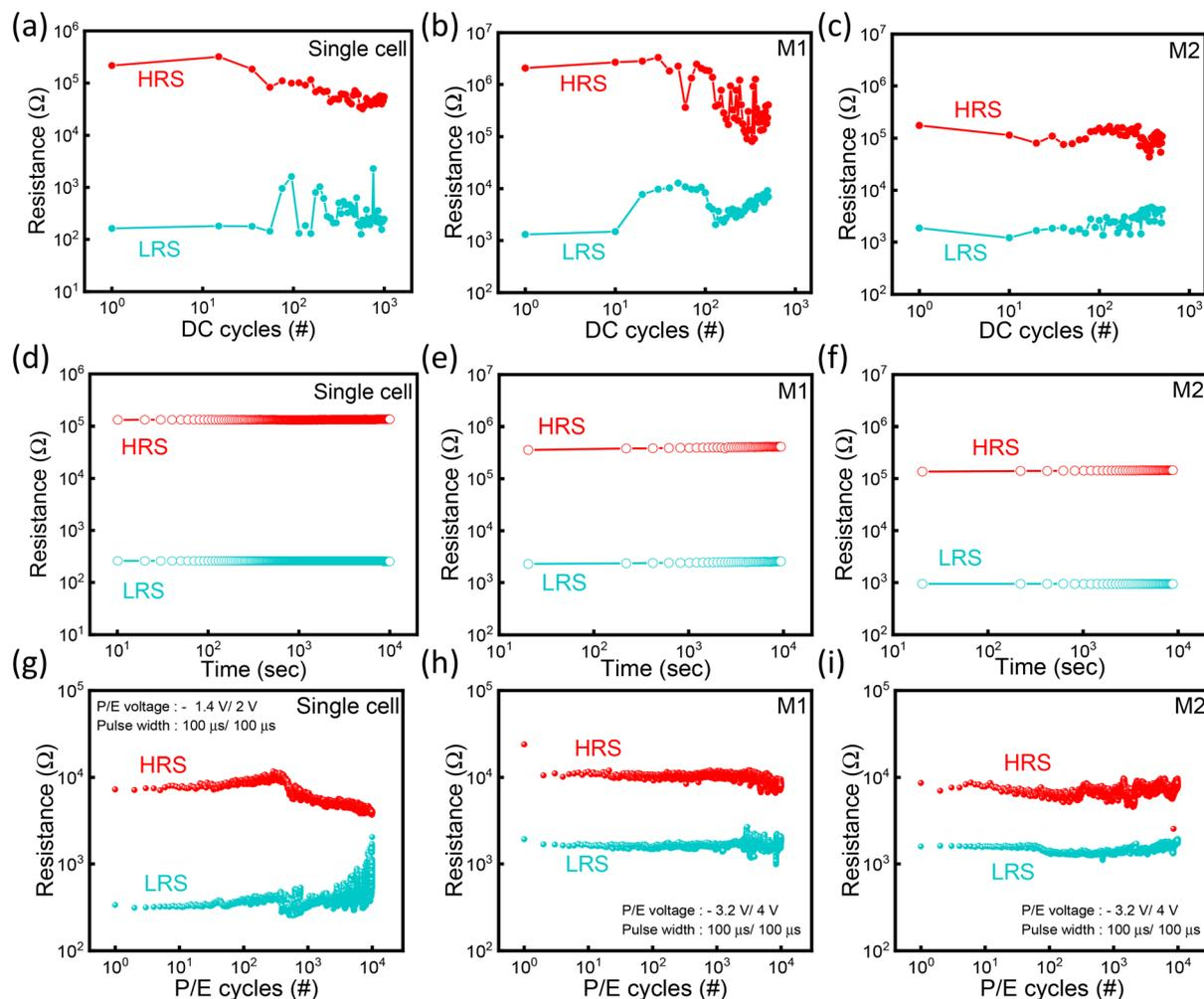
Fig. 5 Endurance characteristics of Pt/Ti/HfO<sub>x</sub>/TiN-NCs/HfO<sub>x</sub>/TiN for (a) a single cell, (b) the first floor (M1), and (c) the second floor (M2) in the HRS and LRS. Retention of three samples measured for 10 000 s: (d) a single cell, (e) M1, and (f) M2 in the HRS and LRS measured at 0.2 V. Pulse endurance: (g) a single cell, (h) M1, and (i) M2.
