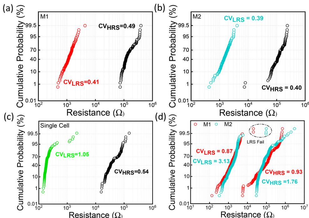
**Fig. 4** Variation of the resistance parameters of four different cells within a device (a) on the first floor (M1) and (b) on the second floor (M2) from 30 consecutive cycles, and (c) five cells in a 2D single cell. (d) The resistance state the cumulative probability of fifteen devices of VRRAM (M1 and M2).
