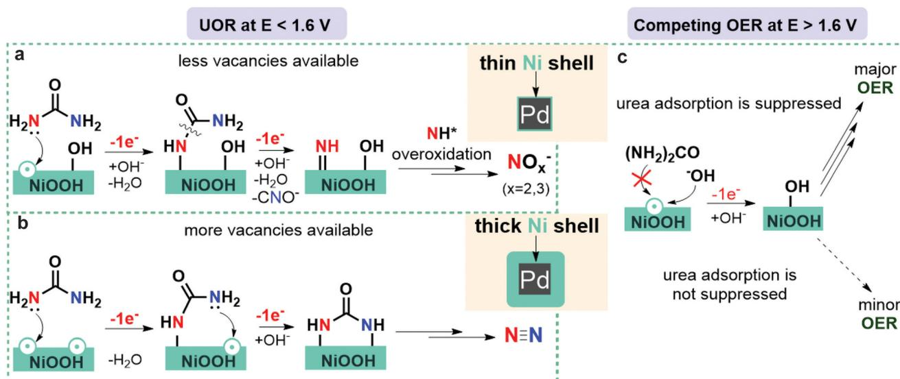
**Fig. 3** The effect of the tensile strain on the UOR mechanistic pathways and competing OER. (a and b) A schematic illustration of the proposed pathways for UOR to  $\text{NO}_x^-$  products (a)  $\text{N}_2$  (b) on the NiOOH surface of Pd@Ni NCs with thin shell (a) and thick shell (b) at  $E < 1.6$  V vs. RHE. (c) A schematic illustration of the competition between UOR and OER on the NiOOH surface of Pd@Ni NCs with thin shell and thick shell at  $E > 1.6$  V vs. RHE.
