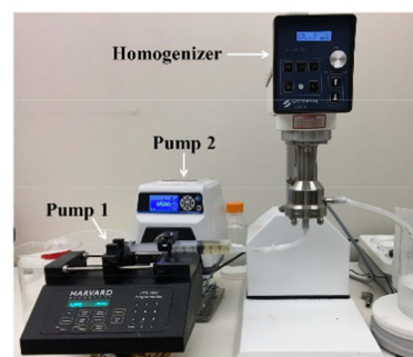
Fig. 6 Utilizing in-line homogenization in the emulsion solvent extraction/evaporation process for producing drug-loaded PLGA particles. (a) Schematic of naltrexone-loaded PLGA generation using an in-line emulsification-extraction process. (b) Experimental set-up used to generate particles by pumping both oil- and aqueous-phases into the homogenizer and transferring the emulsion to the extraction solution. The figure is adopted from ref. 54 with permission.
