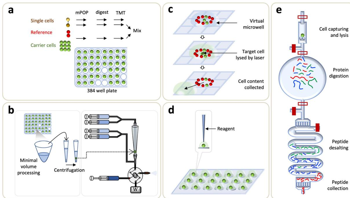
**Fig. 4** Single-cell technologies for non-targeted proteomics. (a) Single-cell proteomics by mass spectrometry (SCoPE-MS). (b) True single-cell-derived proteomics (T-SCP) method. (c) Digital microfluidic based chip. (d) Nanodroplet processing in one-pot (nanoPOTS) chip. (e) Single-cell integrated proteomic microfluidic chip (SciProChip).
