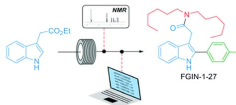
**Scheme 8** Continuous flow synthesis of FGIN-1-27 enabled by in-line <sup>19</sup>F NMR analyses and optimization algorithms. Copyright 2021 Royal Society of Chemistry.<sup>84</sup>
