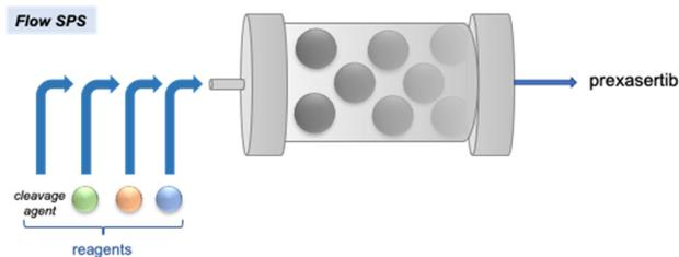
**Scheme 7** Automated synthesis of prexasertib and derivatives enabled by continuous-flow solid-phase synthesis (SPS).<sup>76</sup>
