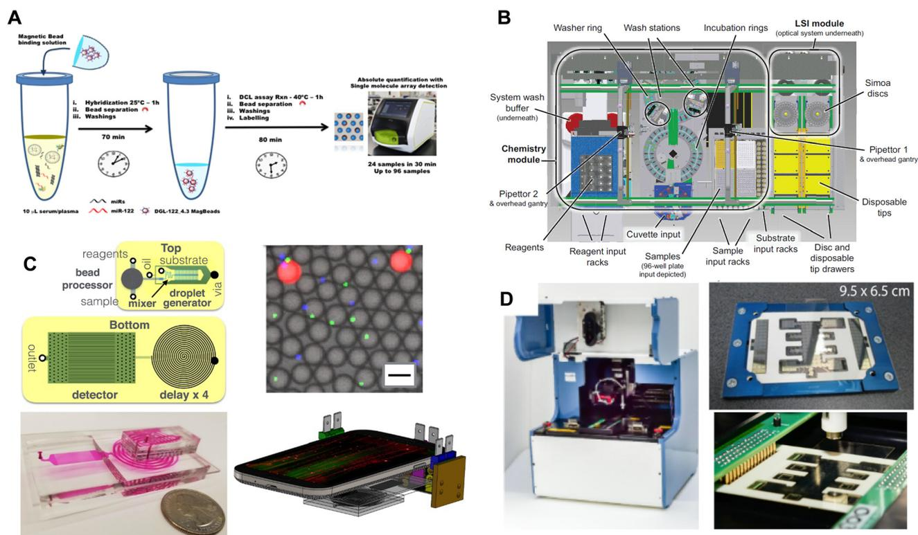
**Fig. 6** Approaches to integrating the assay and single molecule detection steps in DBA. A) Manual pipetting of reagents and automated washing (ref. 90). B) Fully automated system for assays and imaging (ref. 50). C) Miniaturized assay processing based on pressure-driven microfluidics and flow detection on a mobile phone of beads in water-in-oil droplets (ref. 59). D) Miniaturized assay processing based on DMF (ref. 81). Figures reproduced with permissions.
