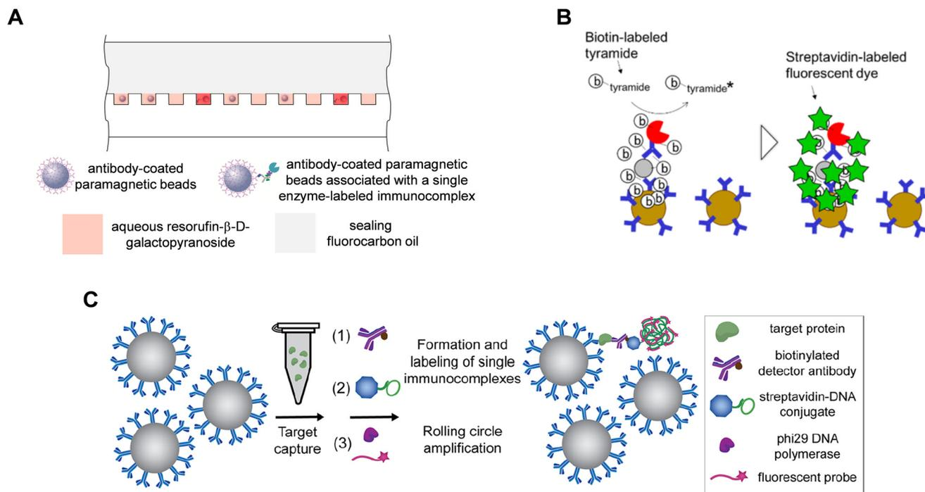
**Fig. 3** Approaches to detecting single molecule labels in DBA. A) Sealing of enzyme-labeled beads with diffusible substrate in arrays of microwells (ref. 55). B) Fluorescent labeling of proteins on beads via tyramide signal amplification (TSA) (ref. 60). C) Formation of DNA concatemers on beads using rolling circle amplification (RCA) followed by labeling with complementary fluorescent probes (ref. 63). Figures reproduced with permissions.
