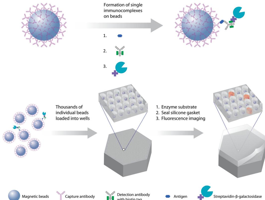
**Fig. 2** The first digital bead assay, based on sealing of beads associated with one or zero immunocomplexes in arrays of microwells, and counting of individual enzyme labels. The method has also become known as digital ELISA and the underlying technology as single molecule arrays (Simoa) (ref. 8). Figure reproduced with permission.
