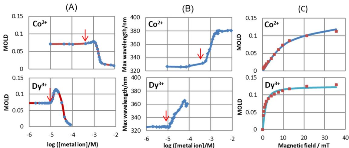
**Fig. 14** Effect of metal ion concentrations of  $\text{Co}^{2+}$  and  $\text{Dy}^{3+}$  on (A) max. MOLD values and (B) max. wavelength of MOLD spectra (35.6 mT). The red arrows show the critical association concentrations. (C) Langevin analysis in  $[\text{Co}^{2+}] = 9.24 \times 10^{-4}$  M and  $[\text{Dy}^{3+}] = 1.67 \times 10^{-5}$  M, 0.00165 wt% MNPs. Reproduced with permission from ref. 205. Copyright © 2020, the American Chemical Society.
