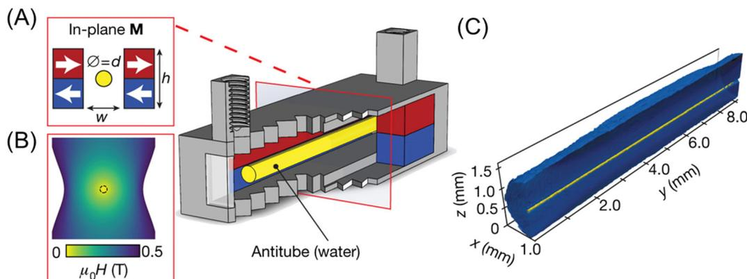
**Fig. 5** (A) Permanent magnets (red, blue) in an in-plane quadrupolar configuration. The yellow area shows a low-field zone created at the centre, where an antitube of water is stabilized inside an immiscible magnetic liquid. (B) Contour plot of the magnetic field. (C) Synchrotron X-ray tomographic reconstruction of a water antitube (yellow) with a diameter of 81  $\mu\text{m}$ , surrounded by ferrofluid (blue). Reproduced from ref. 73 with permission. Copyright © 2020, Springer Nature.
