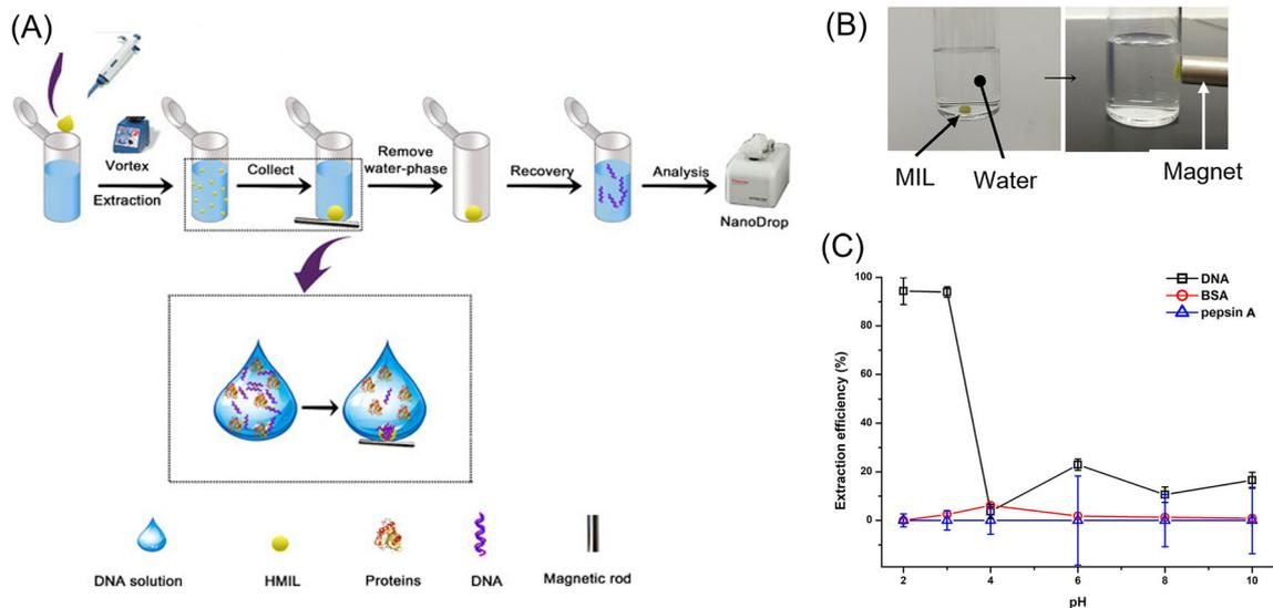
**Fig. 9** Scheme of the extraction procedure (A), attractive behavior of an MIL droplet in water to a magnet (B), and extraction efficiency of stDNA, BSA, and pepsin A as a function of pH (C) for demonstration of the performance of the DNA extraction from complex samples. Reprinted with permission from ref. 135. Copyright © 2021, the American Chemical Society.
