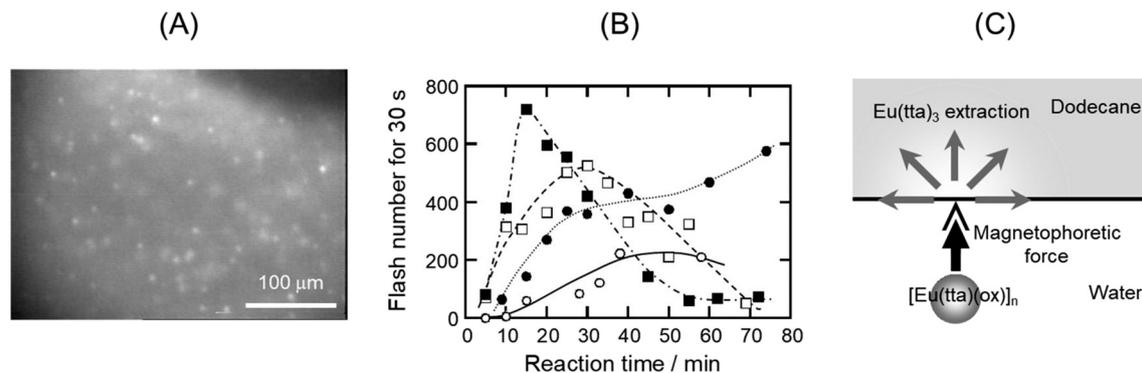
**Fig. 10** (A) Random fluorescent flashing at the dodecane/water interface, showing the extraction of  $\text{Eu}(\text{tta})_3$ . (B) Increase in the extraction rate of  $\text{Eu}(\text{tta})_3$  with a magnetic field; ○ no magnets, ● 2 magnets, □ 6 magnets, and ■ 8 magnets. (C) Illustration of the magnetophoresis of the micro-aggregates of  $[\text{Eu}(\text{tta})(\text{ox})]_n$ . Reprinted from ref. 140.
