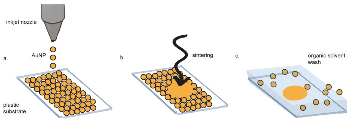
**Fig. 3** Inkjet printed electrode fabrication. (a) Gold nanoparticles (AuNPs) are inkjet printed onto a substrate. (b) The AuNPs are sintered to form a continuous surface. (c) Excess AuNPs are washed away. Figure adapted from ref. 62 (Ko *et al.*, 2007).
